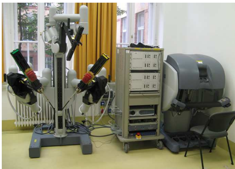
Fig. 6.2. The da Vinci Surgical System and the da Vinci Research Kit. System components: Patient Side Manipulators (left), the DVRK controller (middle) and the Master Tool Manipulators (right).
