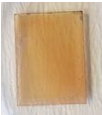
Figure 3.5. Typical appearance of a drop-casted [\text{Fe}^{\text{III}}\text{Cl}_2(\text{tia-BAI})]/\text{ITO} sample [193].
