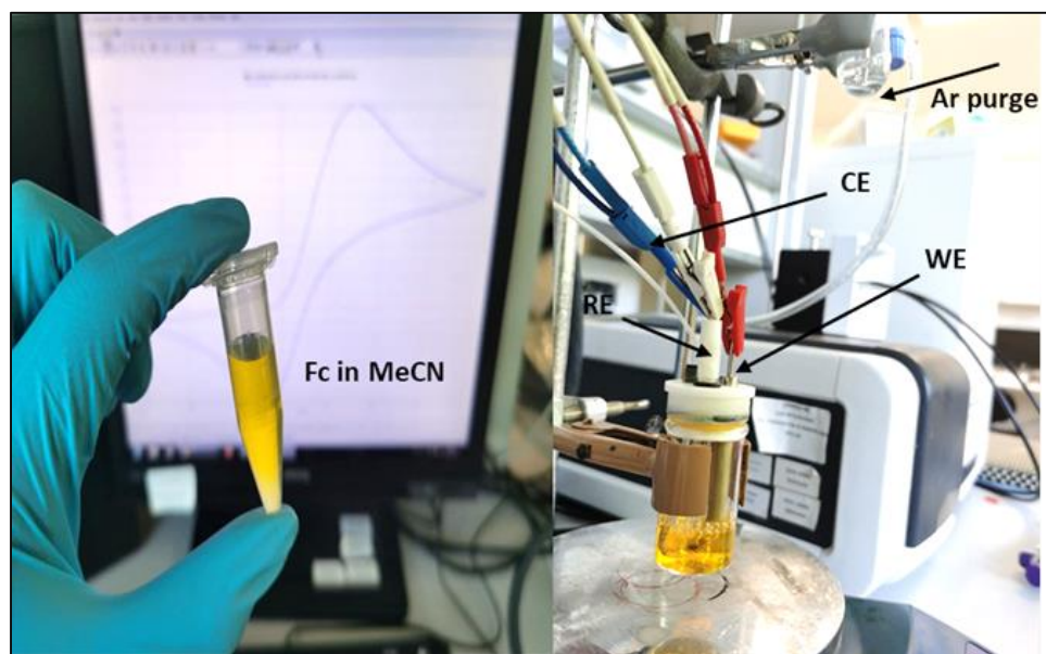
Figure 3.1. Electrochemical cell, three-electrode setup as used in my experimental work.
