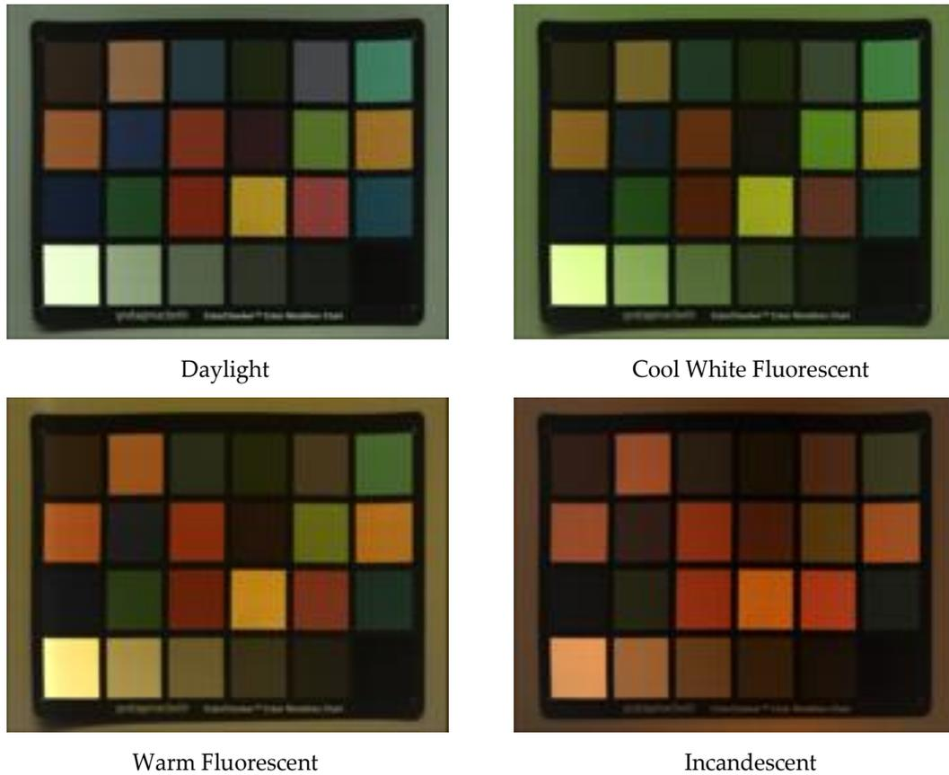
Figure 52: Lens corrected sensor images with different illuminants before color calibration
