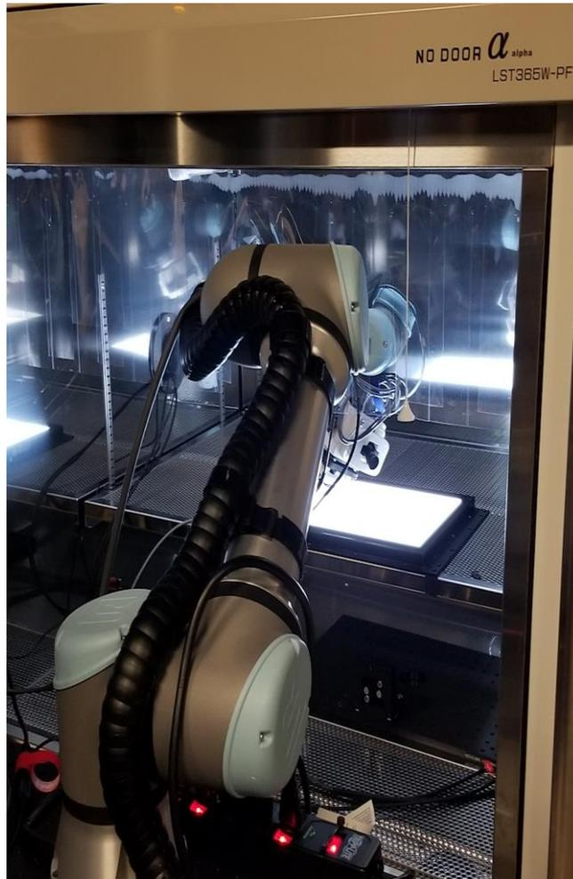
Figure 23 Sensor assembly positioned by articulated robot arm in temperature chamber
