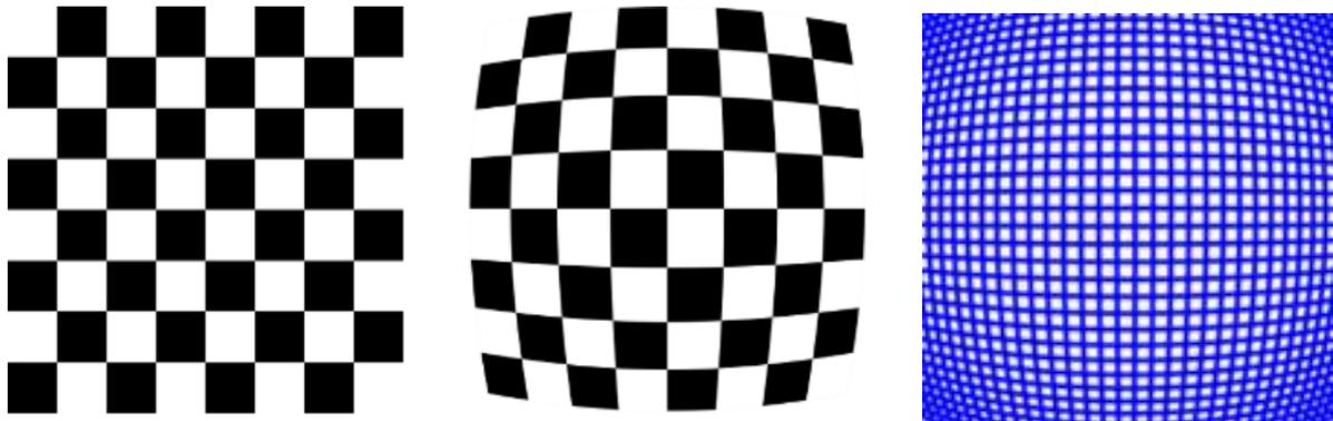
Figure 10: positive radial distortion (a: calibration pattern, b:barrel distortion, c: model)
