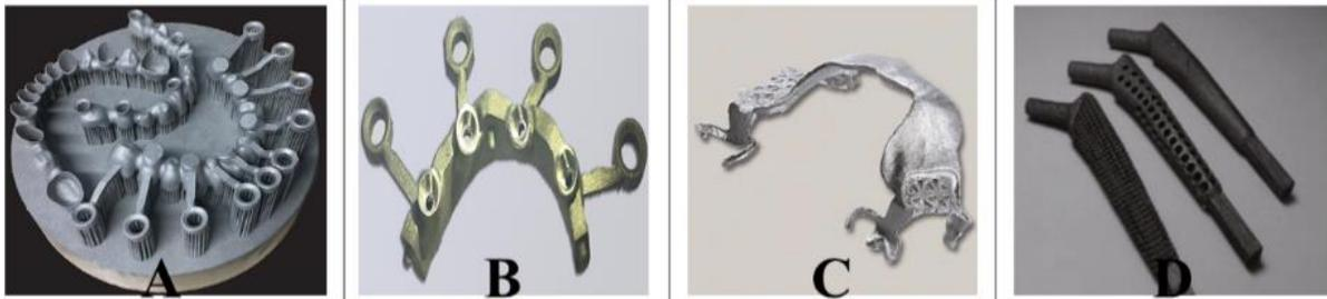
Figure 1-7: Biomedical parts: (a) and (b) Dental prosthesis manufactured by SLM [12], (c) 3-unit dental bridge manufactured by SLM [13], and (d) Hip stems manufactured by EBM [13].
