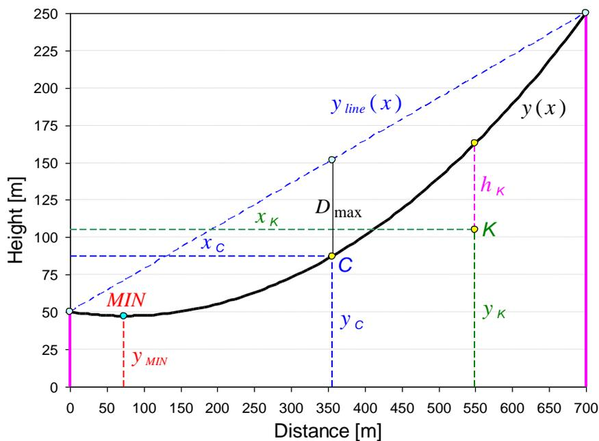
**Fig. 2.8: Conductor curve in Example 2.1**
