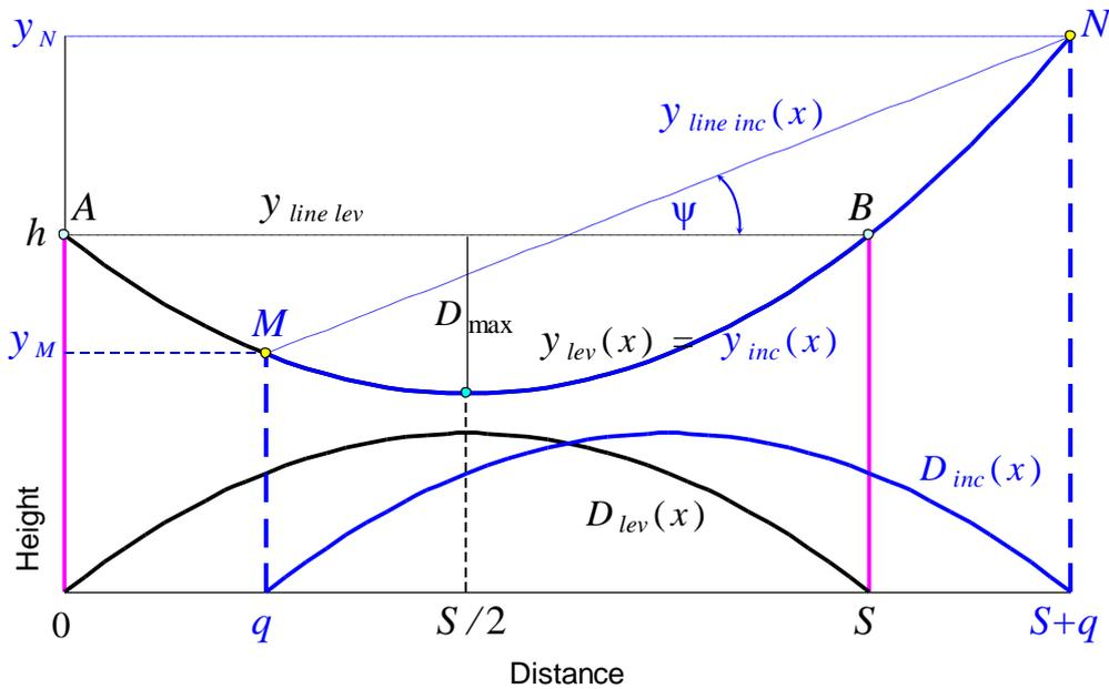
**Figure 4.7: Conductor curves and sag curves in level and inclined spans with the same span length and coefficient  $a$  of the parabola**
