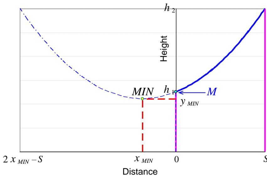
**Fig. 2.6: Special inclined span with  $x_{MIN} < 0$**
