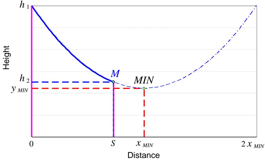
**Fig. 2.7: Special inclined span with  $x_{MIN} > S$**
