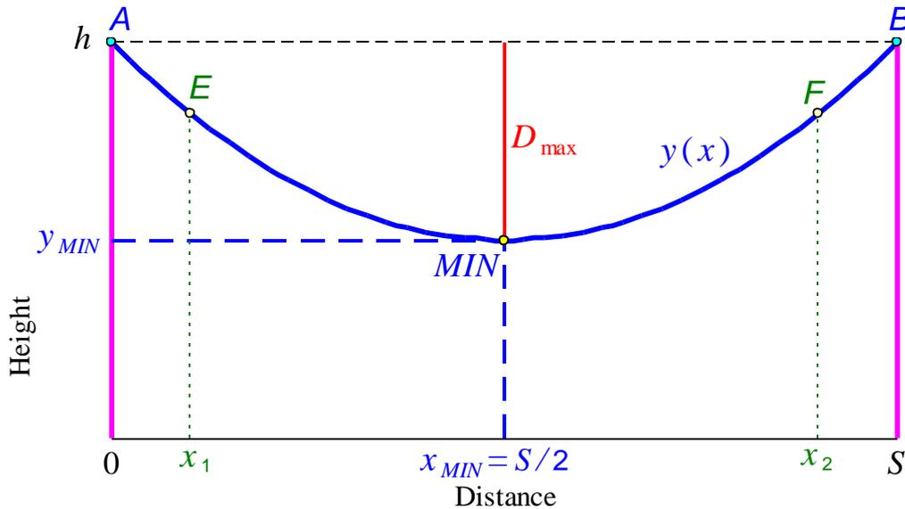
**Fig. 5.2: Parabolic conductor curve in a level span**
