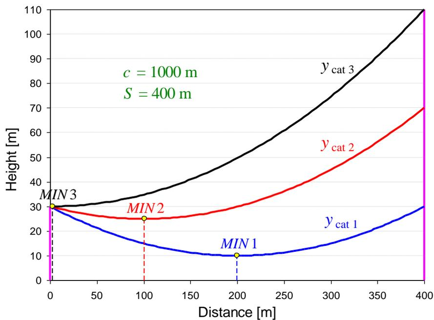
**Figure 4.11: Catenary curves in Example 4.2**
