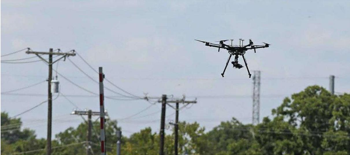
**Fig. 1.13: Overhead line drone inspection [30]**
