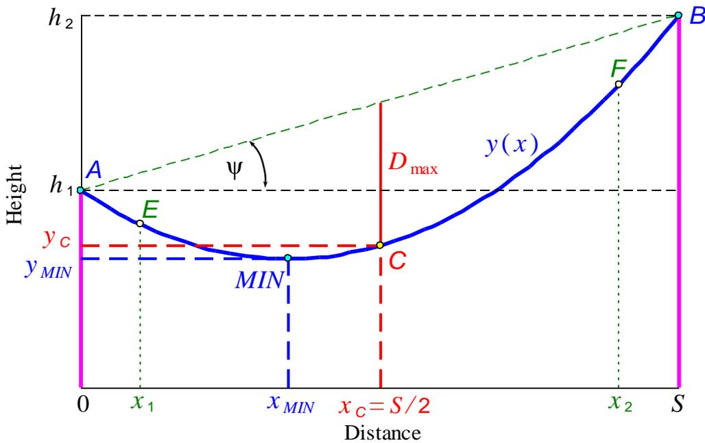
**Fig. 5.1: Parabolic conductor curve in an inclined span with  $h_1 < h_2$**
