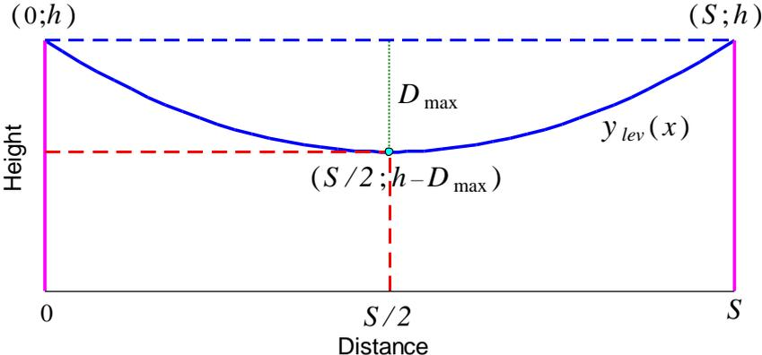
**Fig. 4.4: Conductor curve in a level span**
