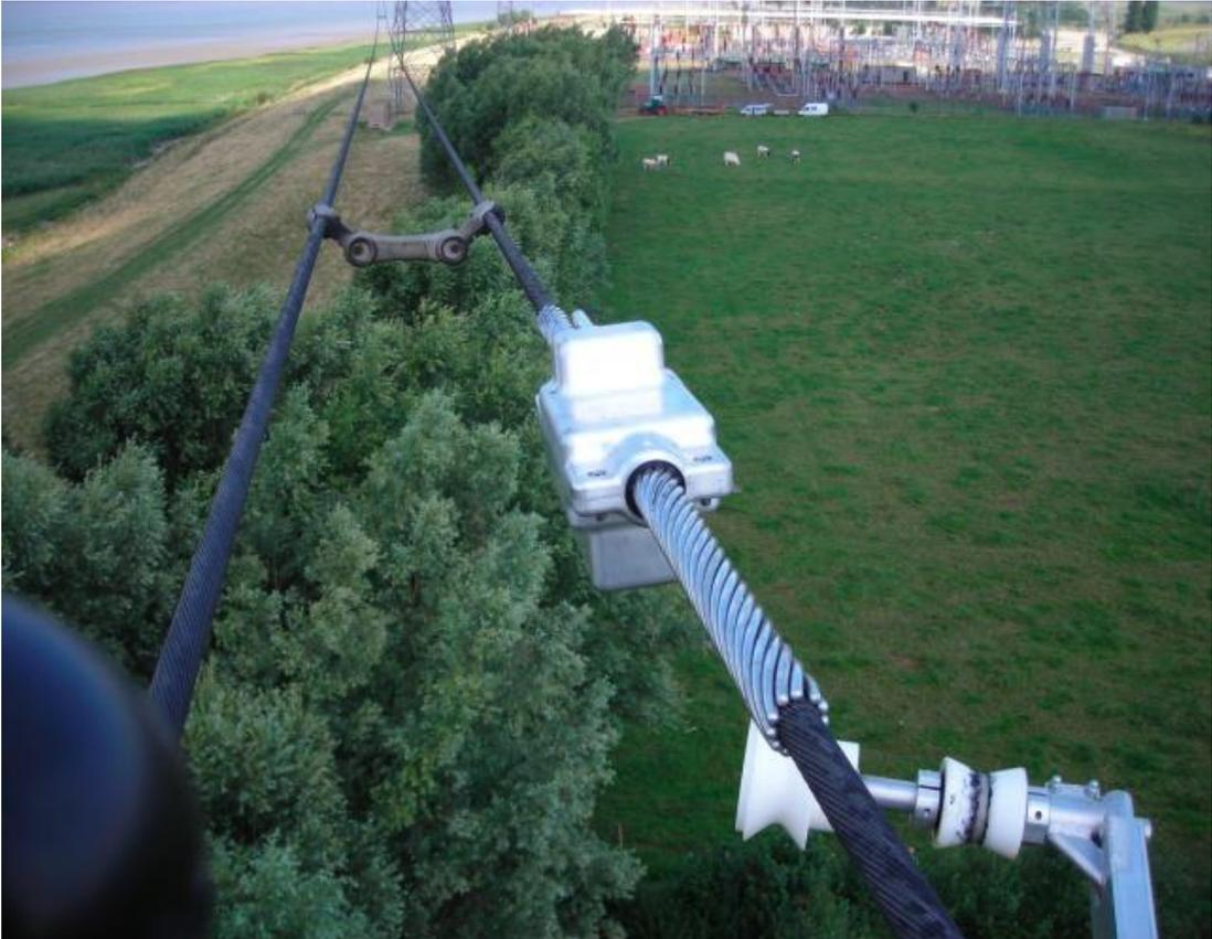
**Fig. 1.12: Sensor for measuring the frequency of the conductor vibrating [24]**
