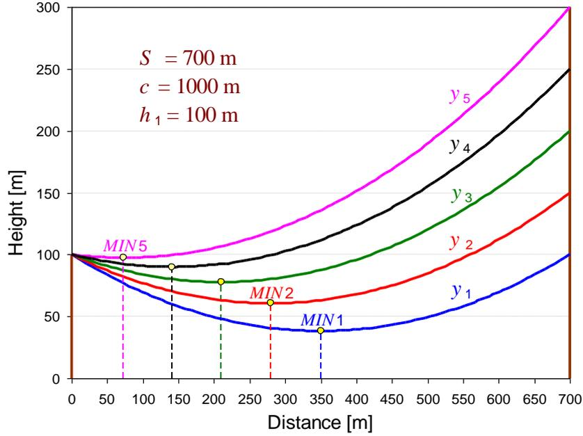
**Fig. 3.11: One curve in a level span and four others in inclined spans**
