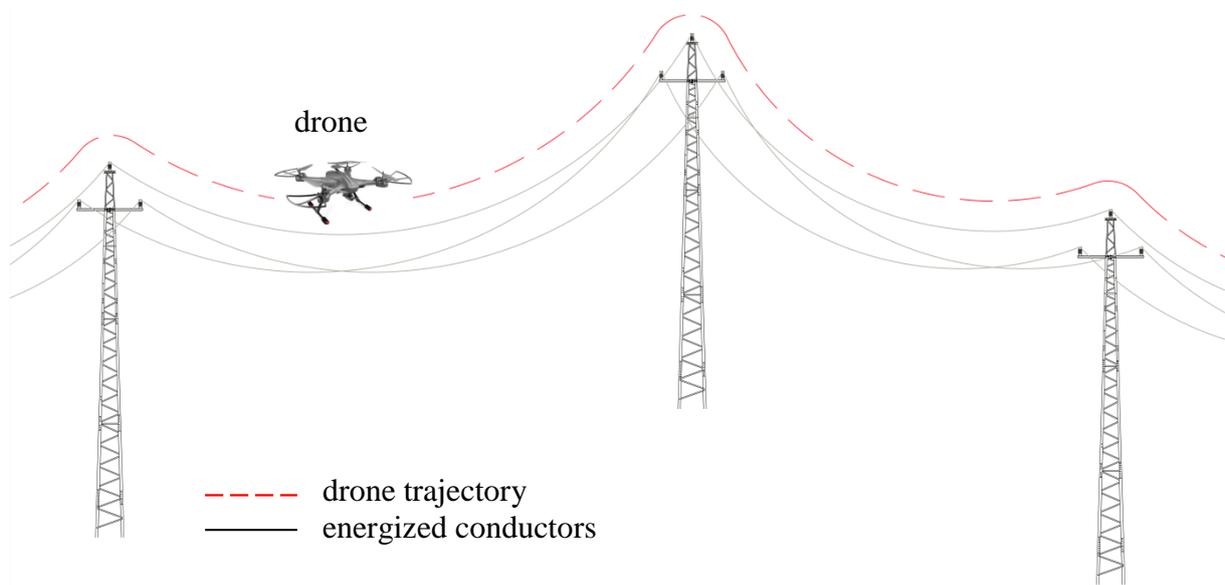
**Fig. 1.2: Principle of overhead line inspection by a drone**
