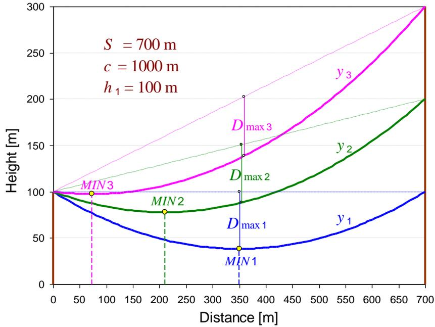
**Fig. 2.10: Conductor curves in Example 2.3**
