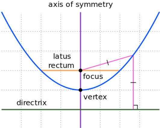
Fig. 4.1: Parabola with various features [70]
