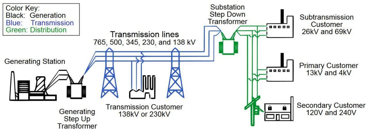
**Fig. 1: The split of elements of electric power global arrangement [2]**
