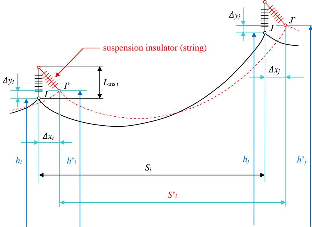
**Fig. 6.1: The  $i^{\text{th}}$  suspension span between the towers  $I$  and  $J$**
