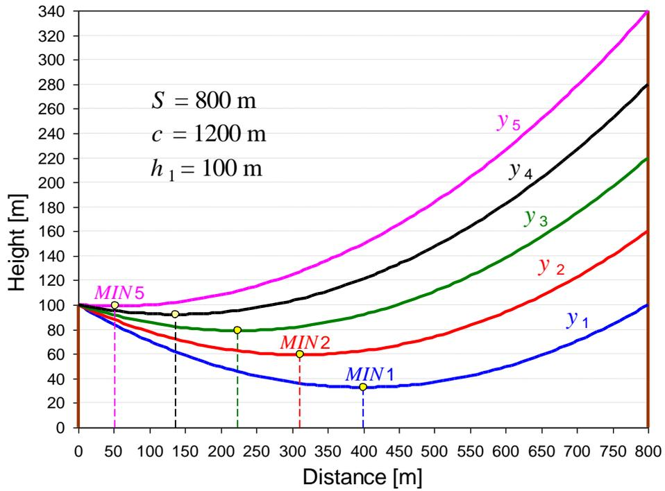
**Fig. 3.5: Conductor curves in Example 3.1**
