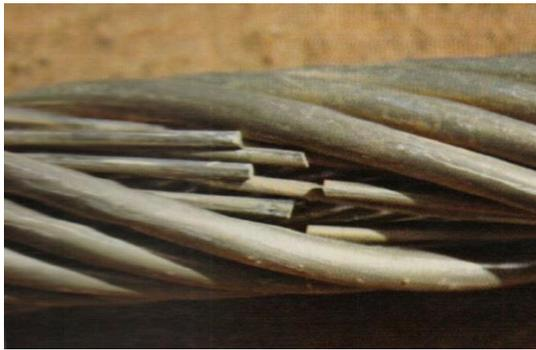
**Fig. 1.10: Strand failure caused by aeolian vibrations [20]**
