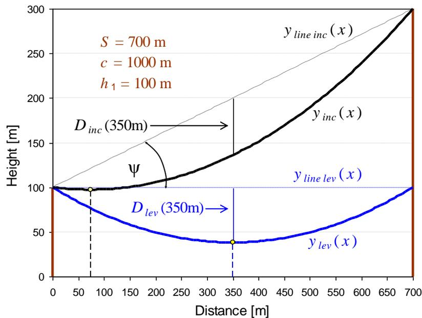
**Fig. 3.9: Conductor curves and mid-span sags in level and inclined spans in Example 3.3**
