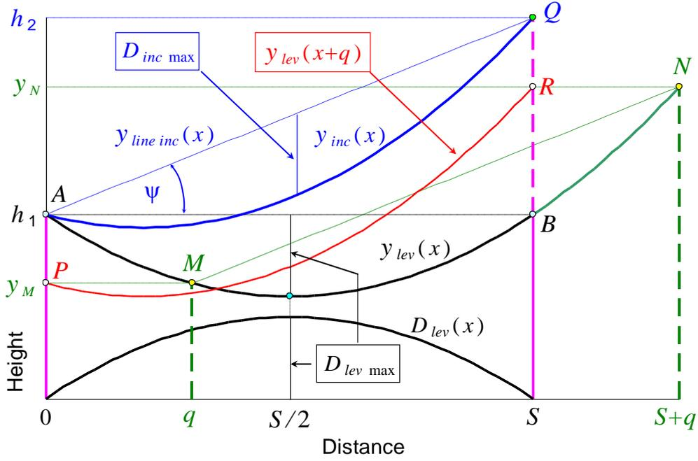
**Fig. 3.4: Curves for explaining the *inclined span modelling by a given level span***
