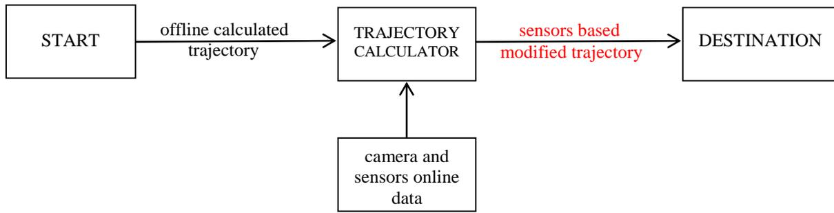
**Fig. 1.3: Combining offline and online planning of a drone trajectory**
