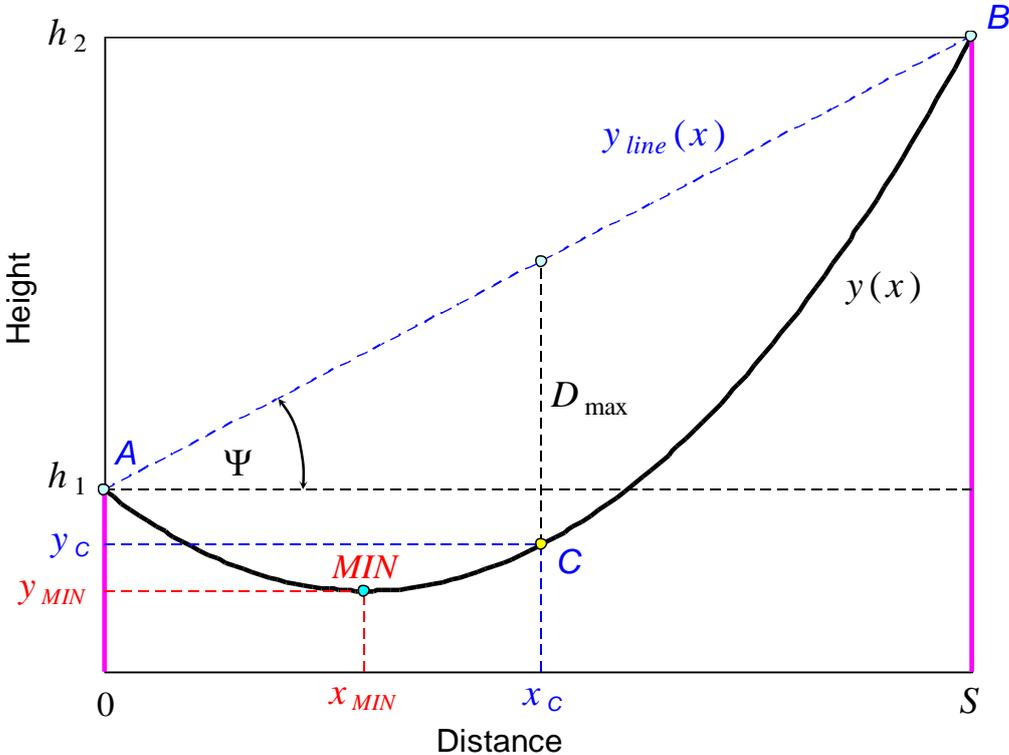
Fig. 2.3: Catenary conductor curve in an inclined span
