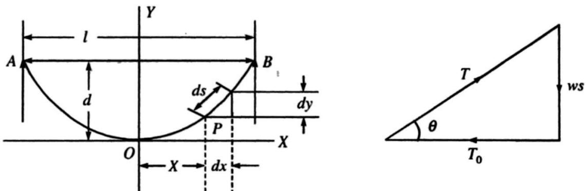
Fig. 2.1: Conductor curve of overhead transmission line [35]
