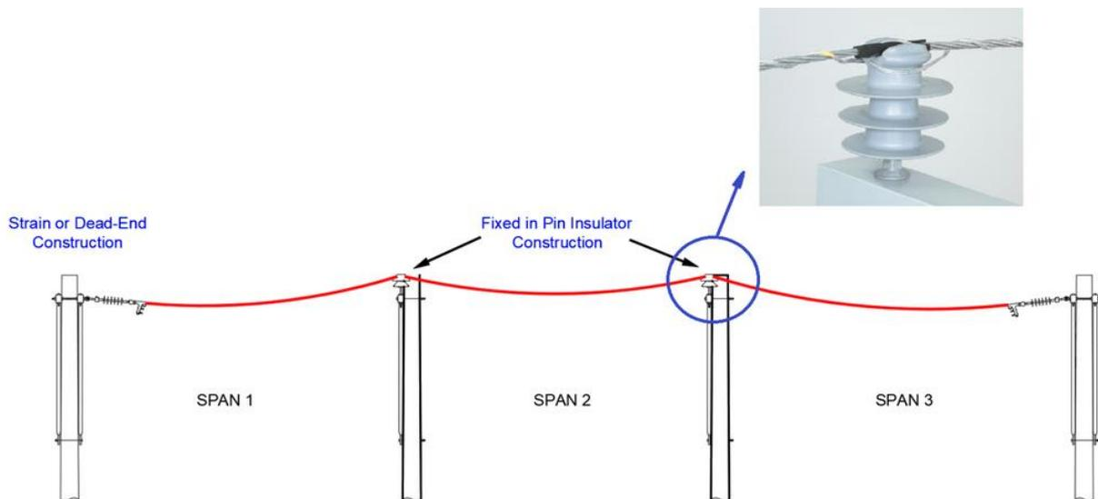
**Fig. 6.2: Mechanically independent spans [105]**
