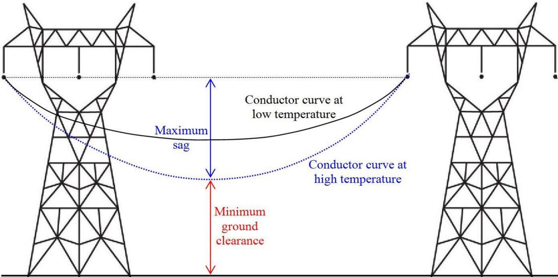
**Fig. 6: Conductor curve, maximum sag and minimum ground clearance**
