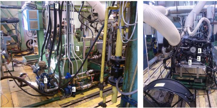
Figure 8: The test rig used for validation (1 - Dynamometer, 2 - 3.0 V6 Diesel engine, 3 - Mounted encoder, 4 - Mounting position of the knock sensor, 5 - KW system, 6 - Intercooler coolant heat exchanger, 7 - Cooling circuit connection)
