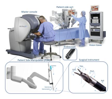
Fig. 3.6. The teleoperational dVSS with the surgeon-side master console, the vision tower and the patient-side cart with the articulated tools of the Patient-Side Manipulators (PSMs). The articulated tool has 6+1 Degrees of Freedom (DoF): insertion, external yaw, external pitch, roll, pitch, yaw and grip. The tools are visualized by an endoscopic camera.
