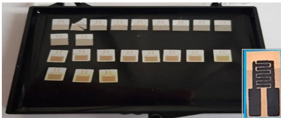
Figure 7-1 Photographs (from different view-angles) of W\text{O}_3/\text{MoO}_3 (lower) or W\text{O}_{3-x}/\text{MoO}_{3-x} (upper) combinatorial sets on heat-able sensor chips. Left hand side is W-rich, and the right one is Mo-rich. No. 6 (middle one) is expected to be 50-50% in both cases. The upper rows show sub-oxides (semi-transparent layers, No. 2 was broken during tweezer handling) the bottom rows show oxides (transparent layers). The inserted photograph shows Pt contacted sample.
