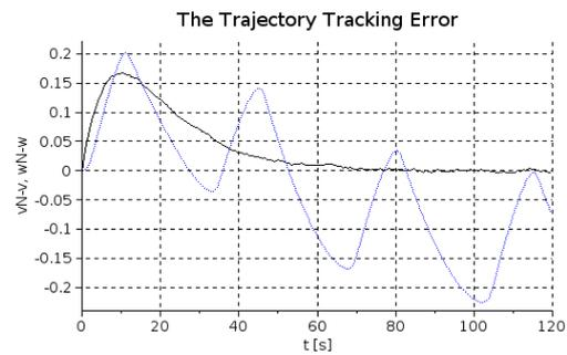
Figure 3.15: Trajectory tracking error for  $v$  in the non-adaptive (LHS) and the adaptive (RHS) cases, under external disturbances:  $v^N - v$ : black solid,  $w^N - w$ : blue dotted lines
