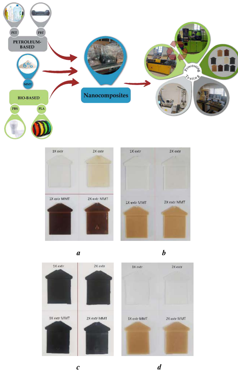
Fig. 36. Injection moulded test specimens: a) PET; b) PBS; c) PBT; d) PLA
